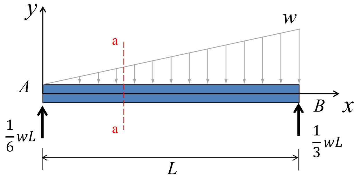
Cut the beam at  $a-a$  to find the moment function  $M(x)$
